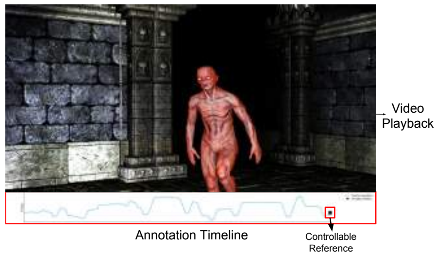
Fig. 5.6 The RankTrace annotation tool. In this example the tool is used for the annotation of tension in horror games. Participants play a game and then they annotate the level of tension by watching a video-recorded playthrough of their game session (top of image). The annotation trace is controlled via a wheel-like user interface. The entire annotation trace is shown for the participant's own reference (bottom of image). Image adapted from [397]. The RankTrace tool is available at: http://www.autogamedesign.eu/software .
